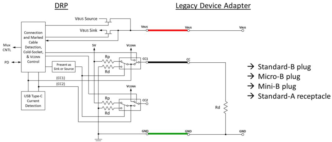
The following describes the behavior when a DRP is connected to a legacy device adapter that has an [Rd](#) to ground so as to mimic the behavior of a Sink.
