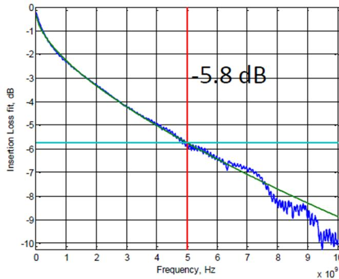
The insertion loss fit at Nyquist frequency ( $IL_{fit@Nq}$ ) shall meet the following requirements:
