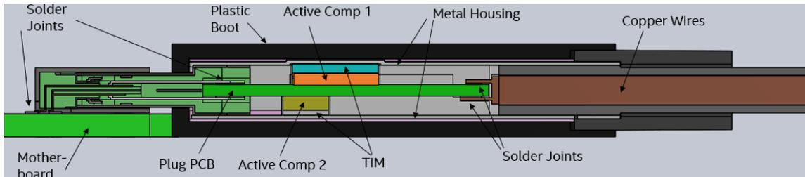
The simplified cable model uses a pure copper cable, representing a typical short active cable, with total cross section of the copper conductors being about 3.8 mm<sup>2</sup>.
