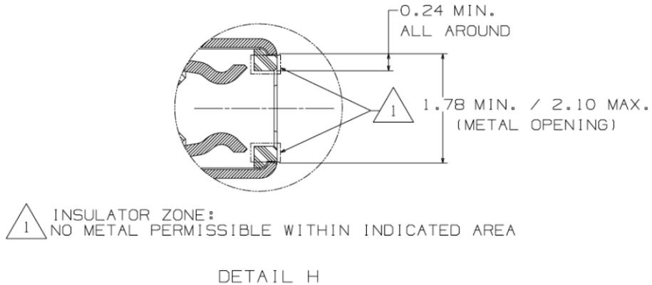
**Figure 3-12 USB Type-C Plug EMC Shielding Spring Tip Requirements**
