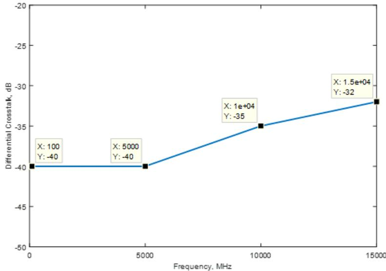
**3.7.2.1.4 Differential Crosstalk between USB D+/D- and TX/RX Pairs (Informative – USB 3.2 Gen2 and USB4 Gen2)**
