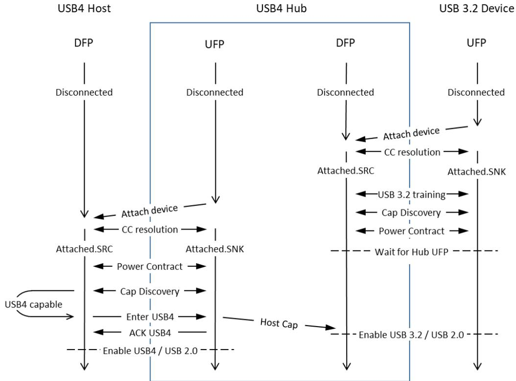
While [USB 3.2](#) devices won't necessarily respond to the Discover ID (SOP), the [USB4](#) hub's DFP will attempt to discover the capabilities of the attached device.
