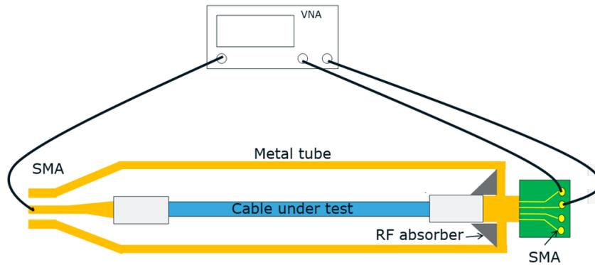
All USB Type-C cable assemblies shall pass the shielding effectiveness test for compliance. Figure 3-65 shows the pass/fail criteria for (a) USB Type-C to USB Type-C cable assemblies, (b) USB Type-C to legacy USB cable assemblies, and (c) the USB Type-C to [USB 3.1](#) Standard-A Receptacle Adapter assembly. Note that the shielding effectiveness for the frequency band from 4 GHz to 5 GHz is not specified since there is no antenna operating in this frequency range.
