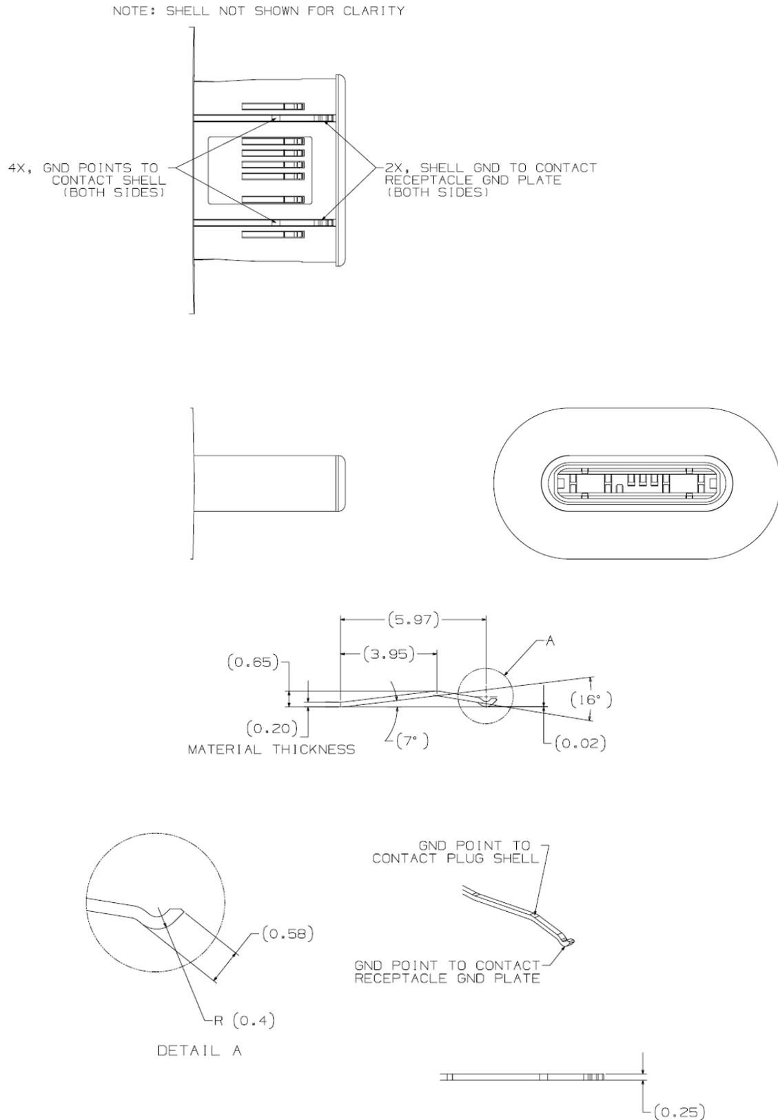
It is critical that the internal EMC spring contacts the plug shell as close to the EMC spring mating interface as possible to minimize the length of the return path.
