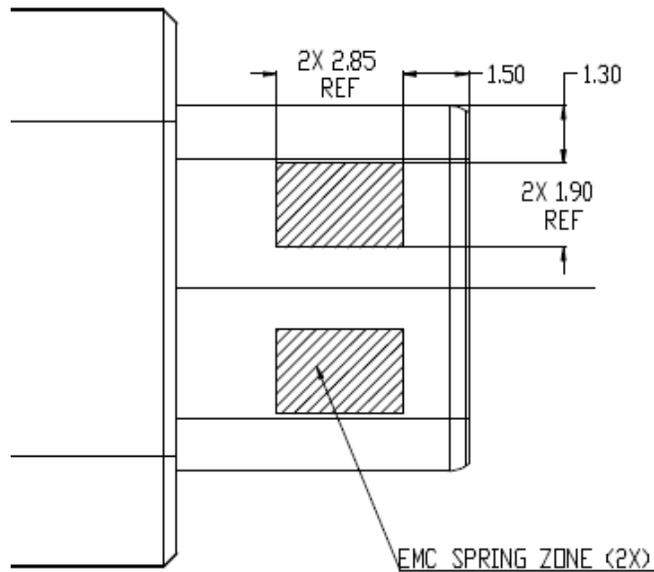
**Figure 3-3 USB Full-Featured Type-C Plug Interface Dimensions**
