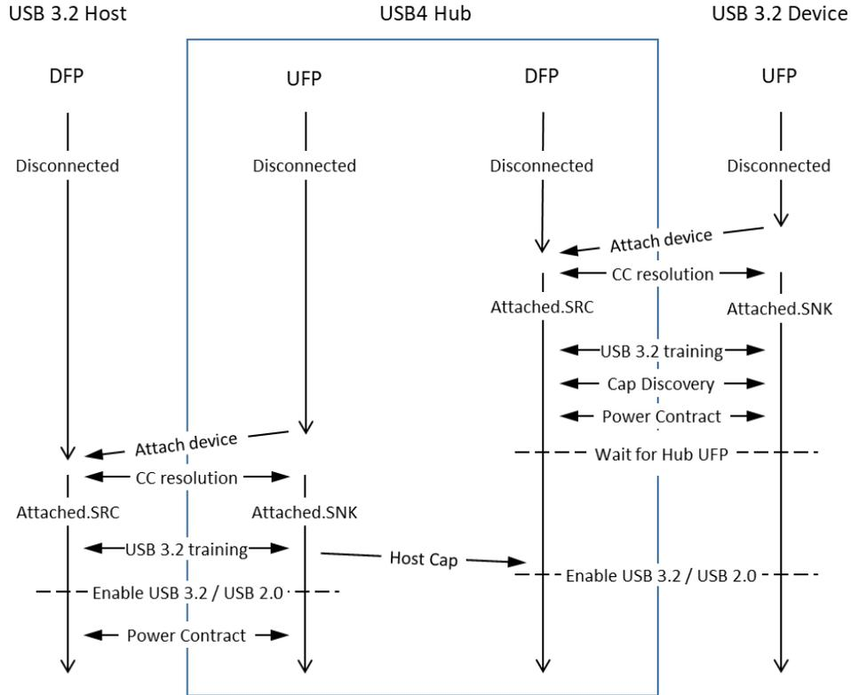
While [USB 3.2](#) devices won't necessarily respond to the Discover ID (SOP), the [USB4](#) hub's DFP will attempt to discover the capabilities of the attached device.
