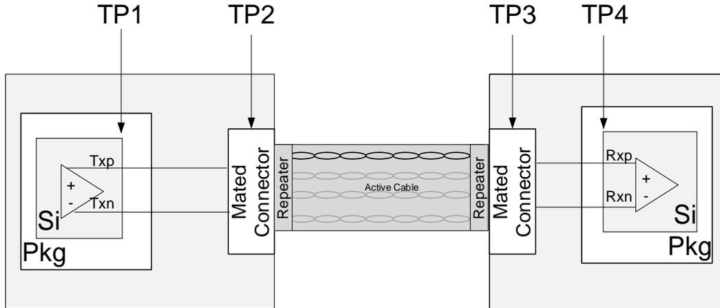
**Figure 6-21 SuperSpeed USB Compliance Test Setup**
