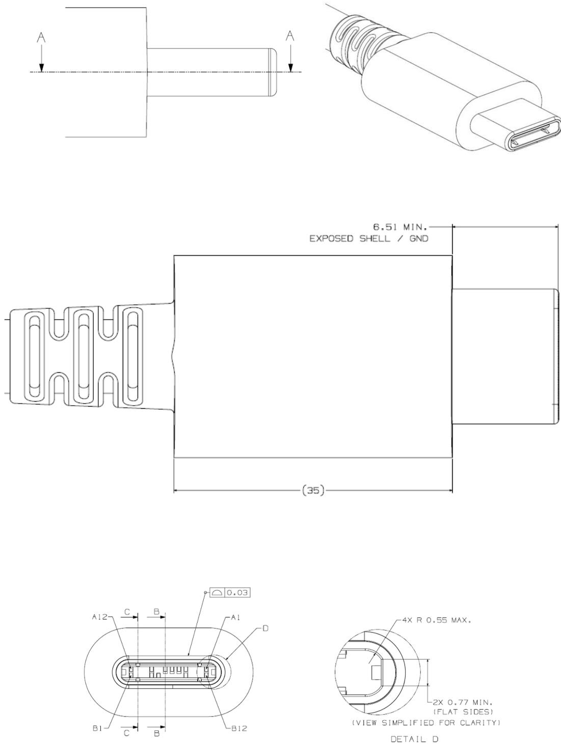
**Figure 3-11 USB 2.0 Type-C Plug Interface Dimensions, cont.**
