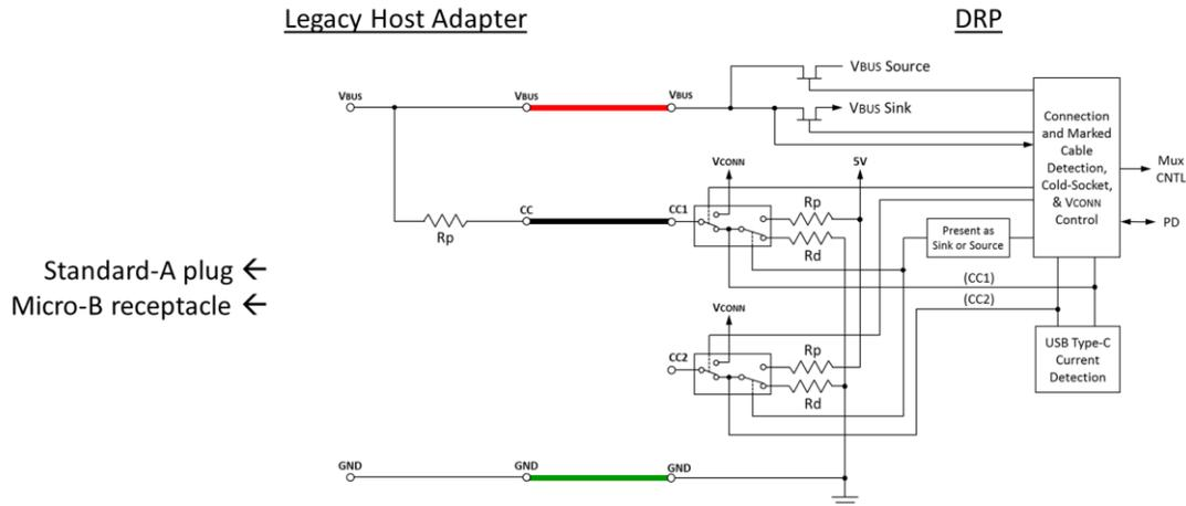
The following describes the behavior when a legacy host adapter that has an [Rp](#) to VBUS so as to mimic the behavior of a Source is connected to a DRP. The value of [Rp](#) shall indicate an advertisement of Default USB Power (See Table 4-24), even though the cable itself can carry 3 A. This is because the cable has no knowledge of the capabilities of the power source, and any higher current is negotiated via [USB BC 1.2](#).
