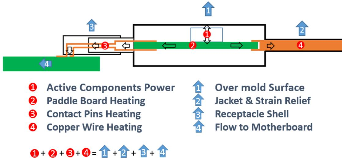
The overall heat generated from the cable should be consistent with the overall power dissipated by the cable. An example of half a 1.0 m active cable consuming 1.5 W and sourcing 5 A  $V_{BUS}$  is shown below:
