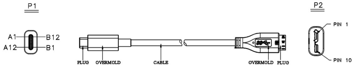
Table 3-17 defines the wire connections for the USB Type-C to [USB 3.1](#) Micro-B cable assembly.
