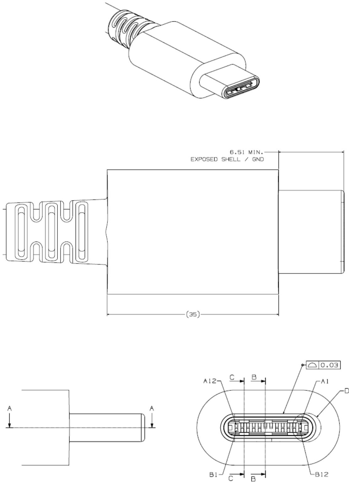
**Figure 3-3 USB Full-Featured Type-C Plug Interface Dimensions, cont.**
