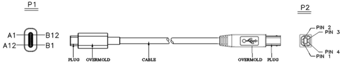
Table 3-15 defines the wire connections for the USB Type-C to [USB 2.0](#) Standard-B cable assembly.
