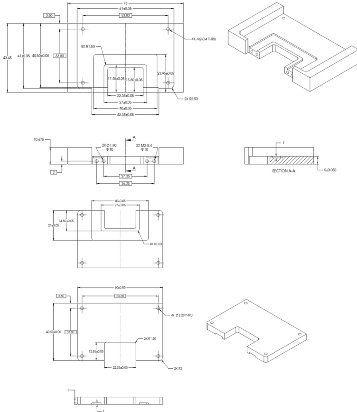
**Figure 3-60 Example of 4-Axis Continuity Test Fixture, cont.**
