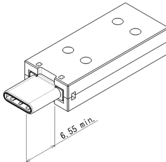
**Figure 3-71 Reference Wrenching Strength Continuity Test Fixture**
