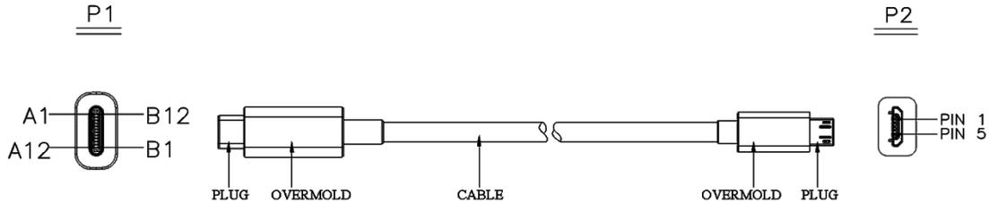
Table 3-18 defines the wire connections for the USB Type-C to [USB 2.0](#) Micro-B cable assembly.
