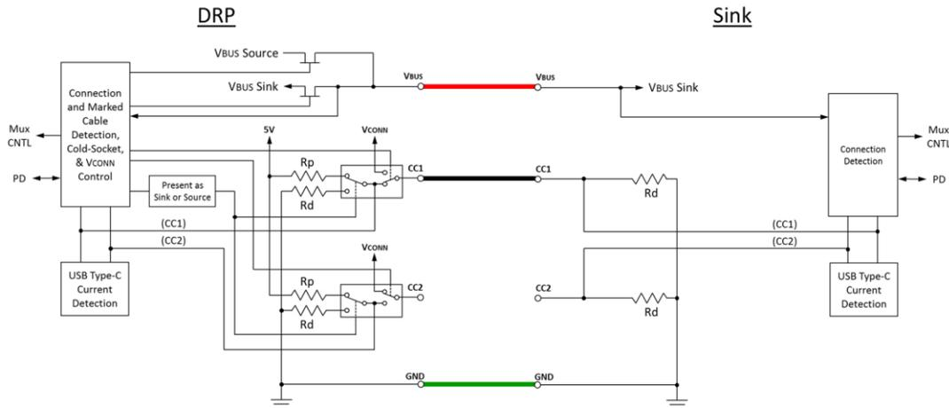
The following describes the behavior when a DRP is connected to a Sink.
