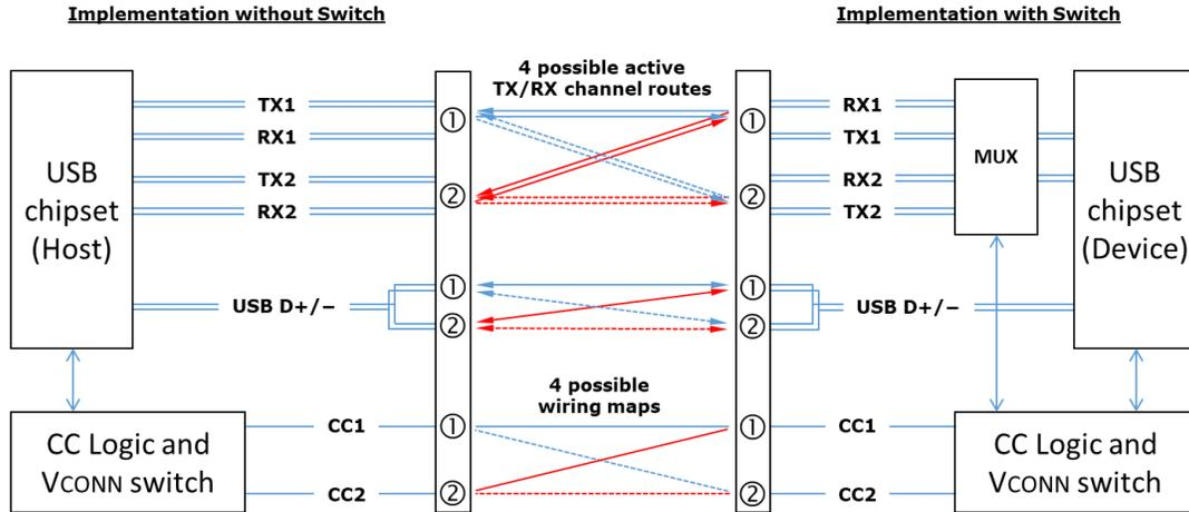
While Figure 4-3 illustrates the functional model as a host connected to a device, this model equally applies to a USB hub's downstream ports as well.
