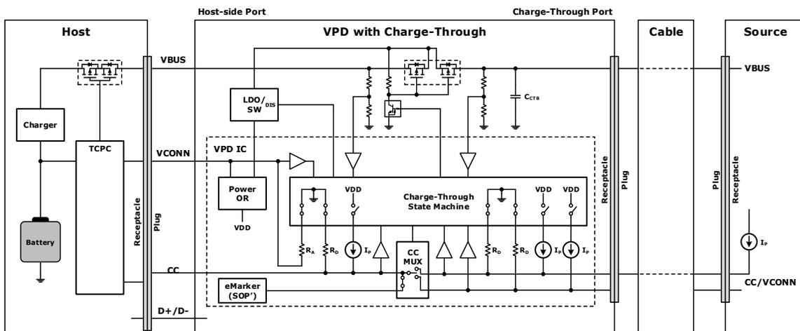
**CASE 1:** The following describes the behavior when a DRP is connected to a Charge-Through [VCONN-Powered USB Device](#) (abbreviated [CTVPD](#)), with no Power Source attached to the Charge-Through port on the [CTVPD](#).
