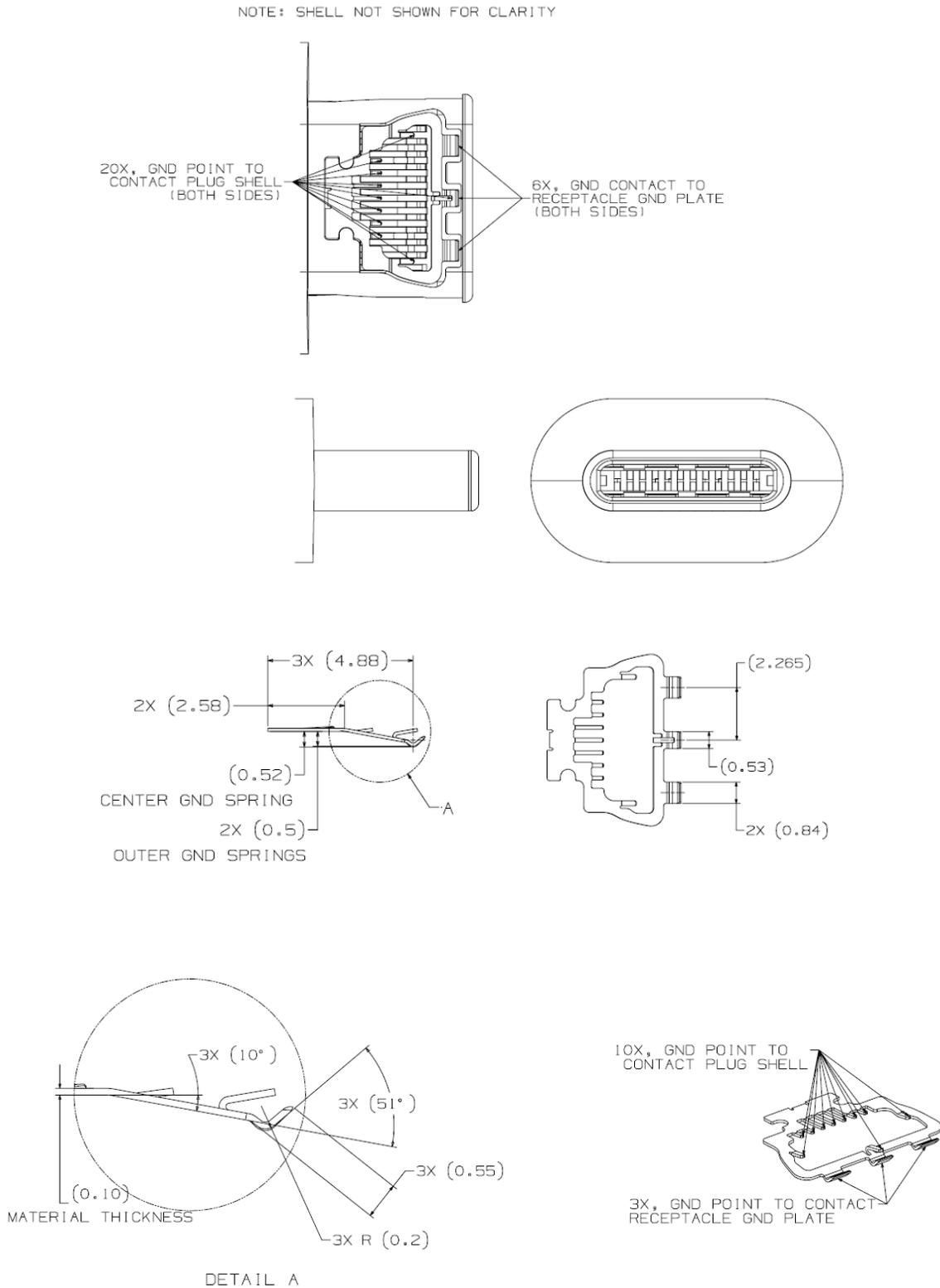
**Figure 3-17 Reference Design of the USB 2.0 Type-C Plug Internal EMC Spring**
