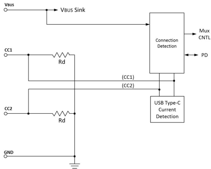
Referring to Figure 4-9, a port that behaves as a Sink has the following functional characteristics:
