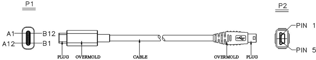
Table 3-16 defines the wire connections for the USB Type-C to [USB 2.0](#) Mini-B cable assembly.
