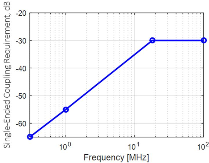
**3.7.2.5.5 Coupling between SBU\_A/SBU\_B and USB D+/D- (Normative)**
