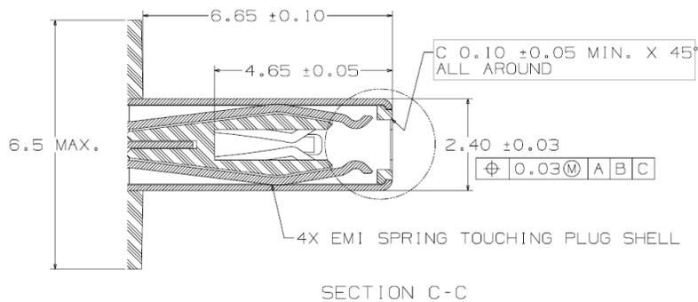
Figure 3-11 **USB 2.0** Type-C Plug Interface Dimensions, cont.
