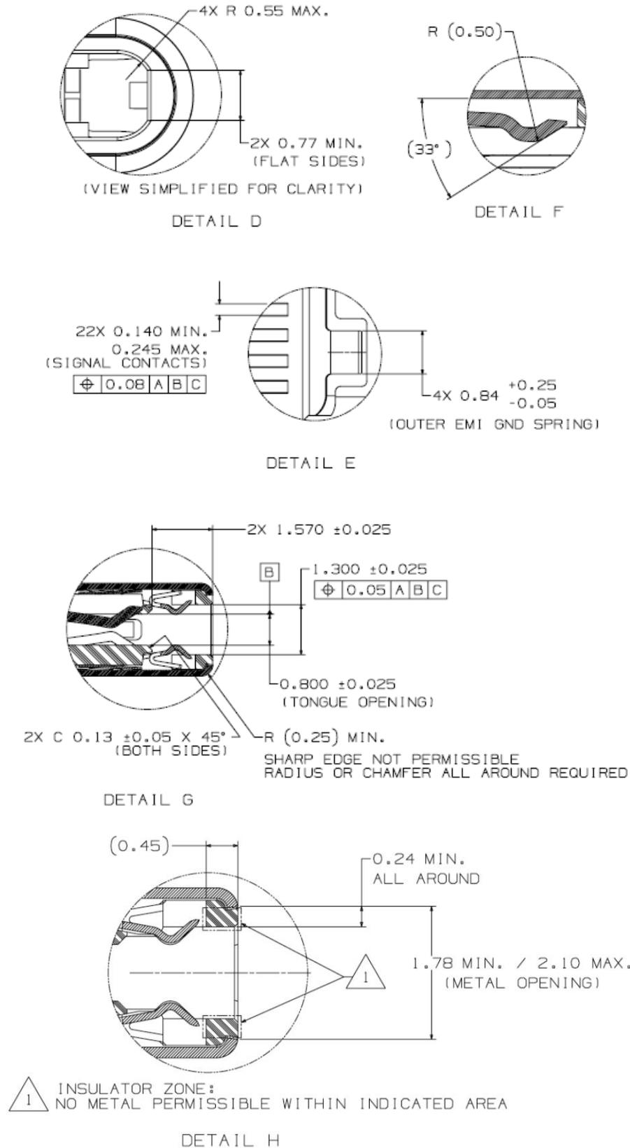
**Figure 3-4 Reference Footprint for a USB Type-C Vertical Mount Receptacle (Informative)**
