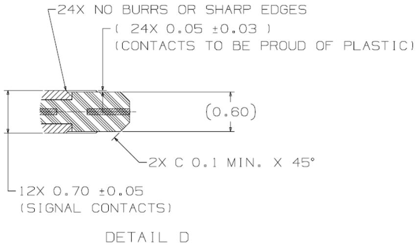
**Figure 3-2 Reference Design USB Type-C Plug External EMC Spring Contact Zones**
