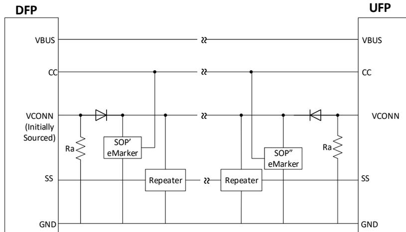
Optically isolated active cables shall be electronically marked on both ends of the cable as illustrated in Figure 6-3
