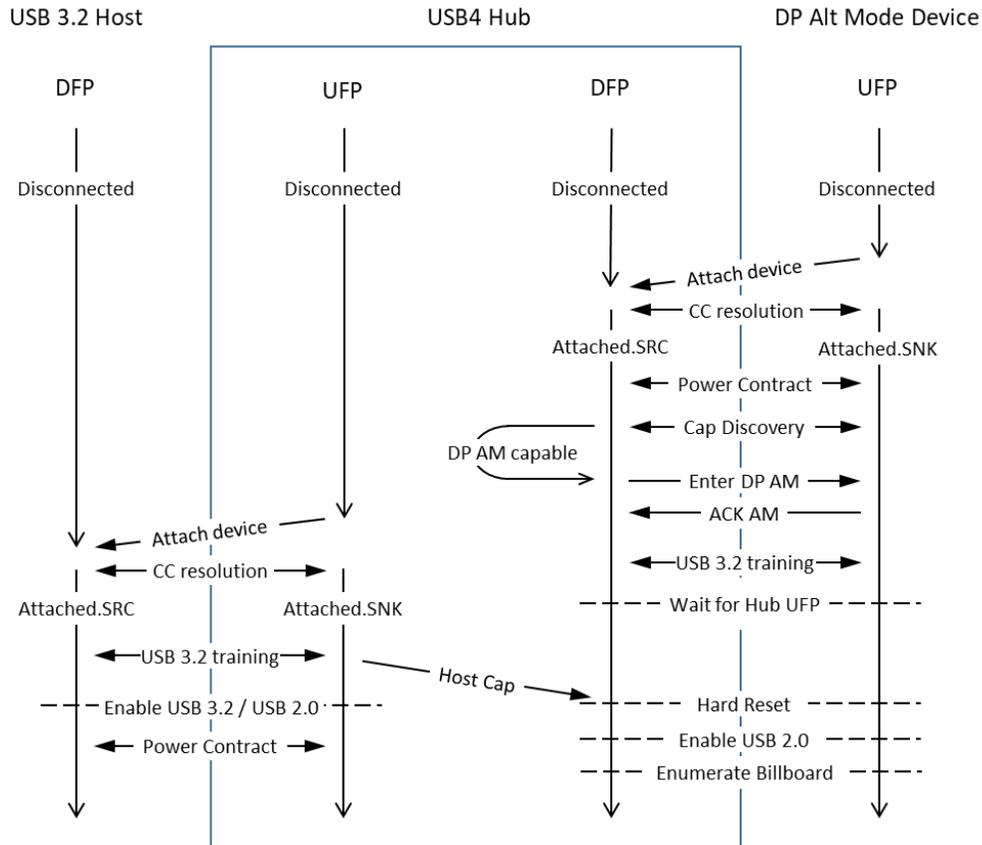
In the flow above, after the [USB 3.2](#) connection of the hub's UFP is established, the DFP connection is no longer valid with the [USB4](#) hub now operating as a traditional [USB 3.2](#) hub. The hub's DFP shall then reset the port which will lead to a [USB 2.0](#) connection and the exposure of the Billboard device.
