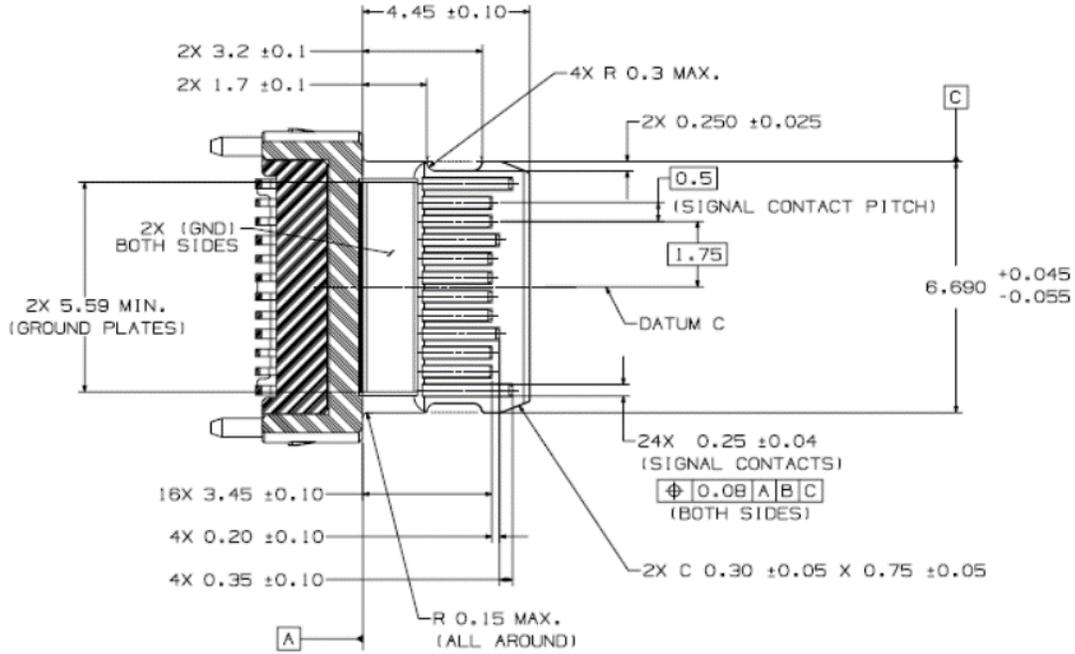
ALTERNATE SECTION A-A dimensions for use if the receptacle shell is non-conductive or there is no receptacle shell. This configuration is also allowed for receptacles with a conductive shell. See text for full requirements.
