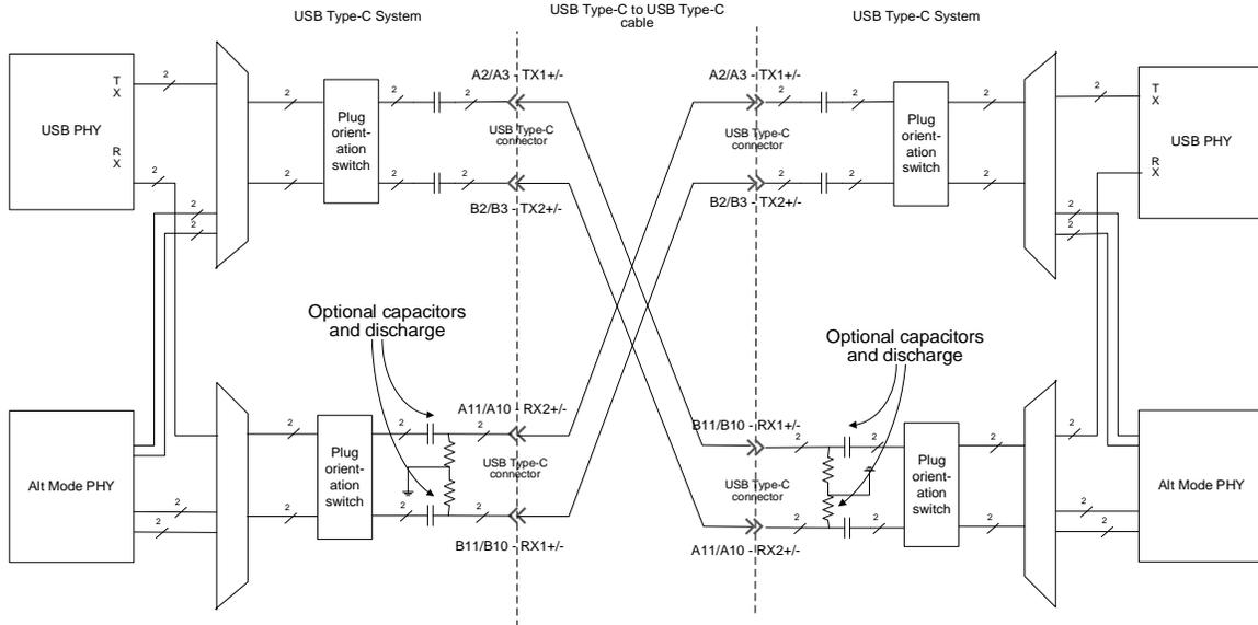
In the case where the Alternate Mode System is required to implement DC blocking capacitors within the system between active system components and the Alternate Mode connector, then this provides the necessary isolation and further capacitors in the USB Type-C to Alternate Mode adapter cable are not necessary, and may indeed impair signal integrity.
