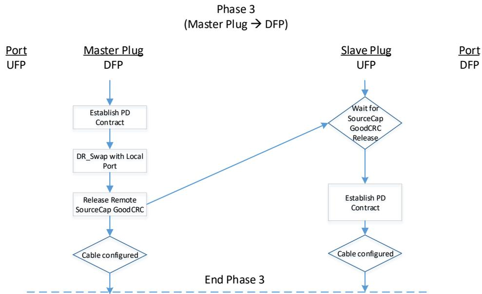
Figure 6-13 OIAC Master Plug Configure as UFP - Phase 3
