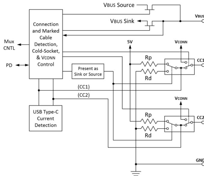
Referring to Figure 4-11, a port that can alternate between DFP and UFP behaviors has the following functional characteristics:
