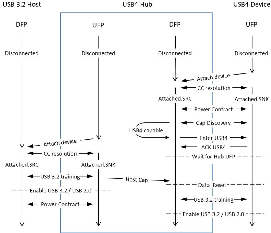
In the flow above, once connected to a [USB 3.2](#) host, the Host Cap reflects that the hub can only support [USB 3.2](#) on its DFPs and the speculatively established [USB4](#) connection on the DFP is exited with the [USB4](#) hub now operating as a traditional [USB 3.2](#) hub.
