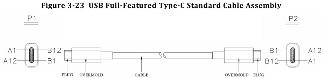
Table 3-10 defines the wire connections for the USB Full-Featured Type-C standard cable assembly.
