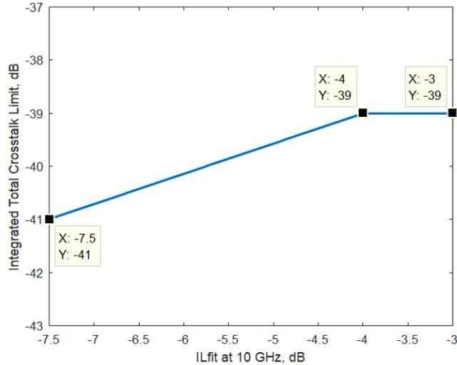
**3.7.2.4.4 Integrated Crosstalk from TX/RX Pairs to USB 2.0 D+/D- (Normative – USB4 Gen3)**
