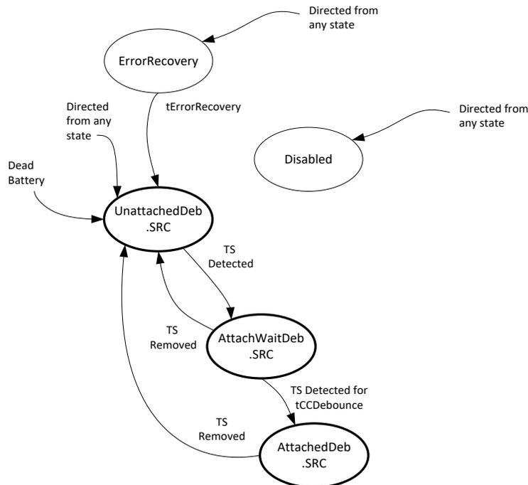
Figure B-5 illustrates a connection state diagram for a DTS DRP.
