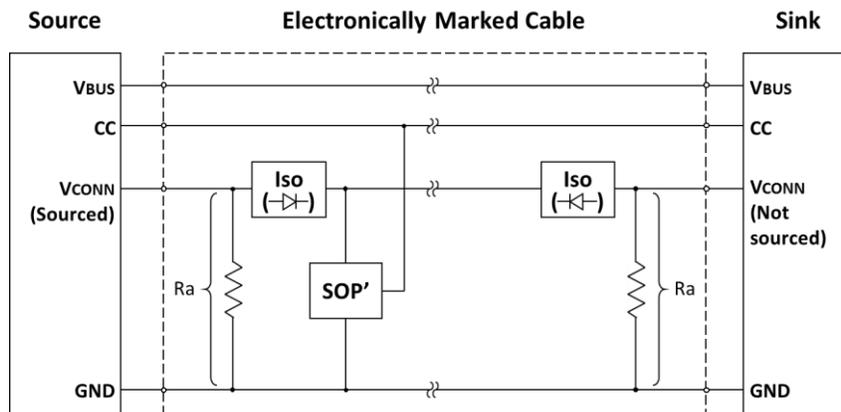
Figure 4-42 illustrates an electronically marked cable where the VCONN wire does not extend through the cable, therefore an SOP' (eMarker) element is required at each end of the cable. In this case, no isolation elements are needed.
