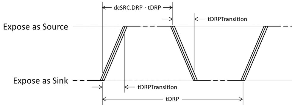
Table 4-30 provides the timing values that shall be met for DRPs. The clock used to control DRP swap should not be derived from a precision timing source such as a crystal, ceramic resonator, etc. to help minimize the probability of two DRP devices indefinitely failing to resolve into a Source-to-Sink relationship. Similarly, the percentage of time that a DRP spends advertising Source not be derived from a precision timing source.
