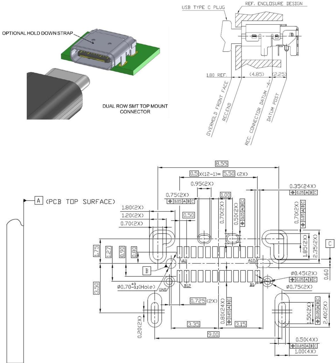
**Figure 3-6 Reference Footprint for a USB Type-C Hybrid Right-Angle Receptacle
