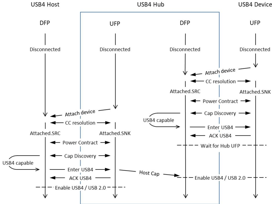
In the illustrated flow, Cap Discovery includes all [USB PD](#) message exchanges needed between the DFP and its UFP port partner to discover the UFP’s USB capabilities along with TBT3-compatibility and DP Alt Mode capabilities. For the [USB4](#) hub’s DFP, Cap Discovery is done on a speculative basis whenever it does not already know of the capabilities of the host that will eventually be connected via the hub’s UFP.
