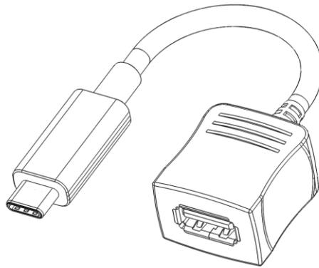
Table 3-19 defines the wire connections for the USB Type-C to [USB 3.1](#) Standard-A receptacle adapter assembly.
