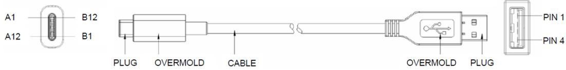
Table 3-13 defines the wire connections for the USB Type-C to [USB 2.0](#) Standard-A cable assembly.
