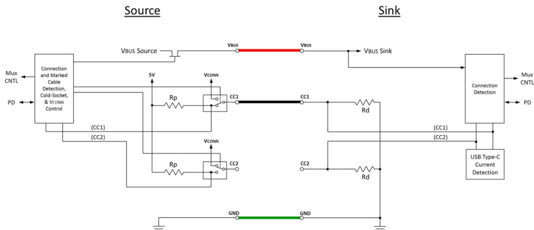
The following describes the behavior when a Source is connected to a Sink.
