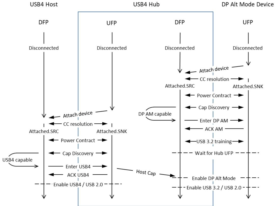
In the flow above, after the [USB4](#) connection of the hub's UFP is established, the DFP connection remains valid with the DisplayPort and [USB 3.2](#) data paths of the DFP being serviced by the [USB4](#) DisplayPort and Enhanced SuperSpeed tunnels.
