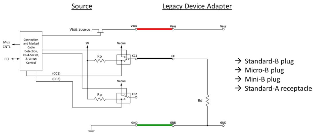
The following describes the behavior when a Source is connected to a legacy device adapter that has an [Rd](#) to ground so as to mimic the behavior of a Sink.
