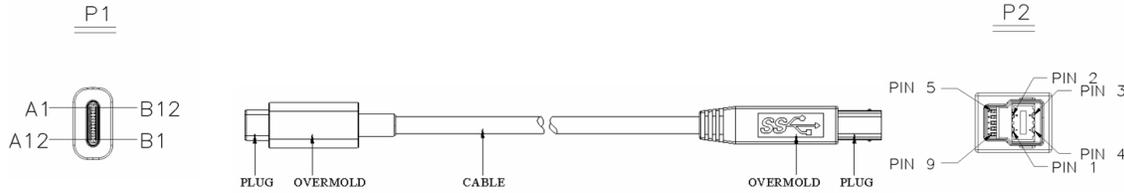
Table 3-14 defines the wire connections for the USB Type-C to [USB 3.1](#) Standard-B cable assembly.
