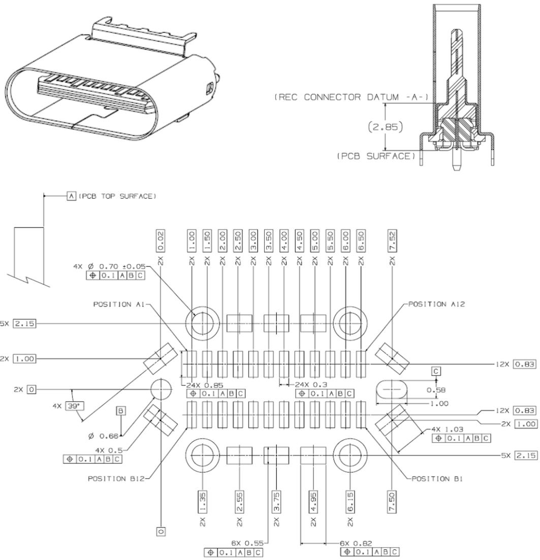
**Figure 3-5 Reference Footprint for a USB Type-C Dual-Row SMT Right Angle Receptacle (Informative)**
