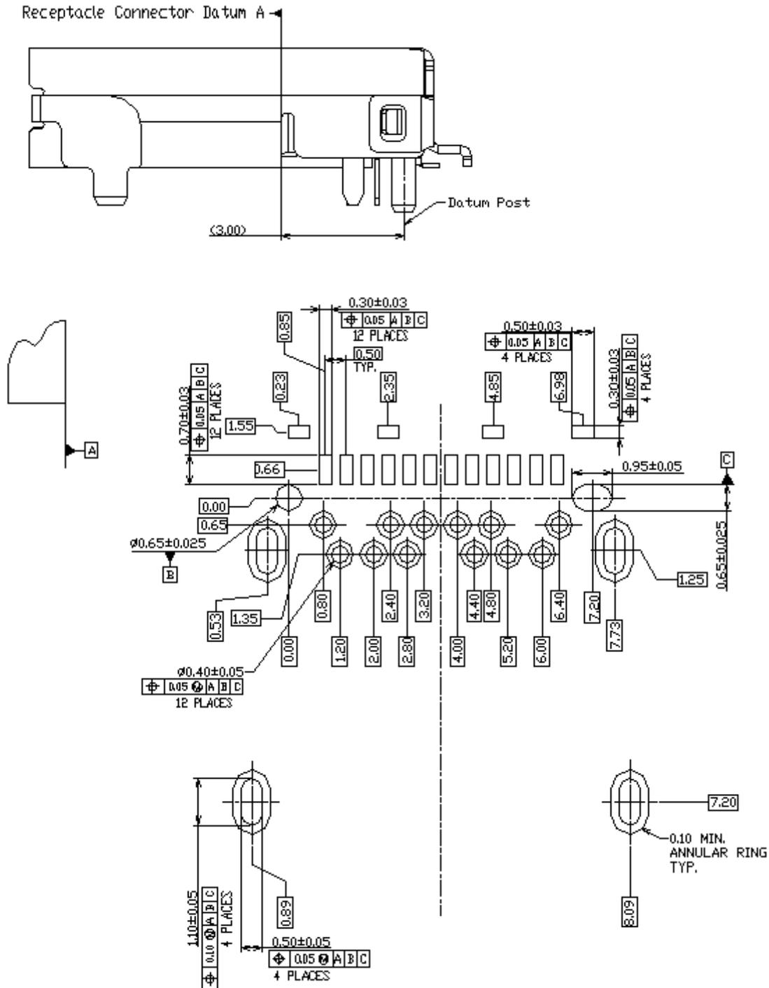
**Figure 3-9 Reference Footprint for a USB 2.0 Type-C Through Hole Right Angle Receptacle (Informative)**
