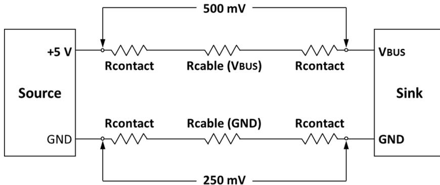
Figure 4-2 illustrates what parameters contribute to the IR drop for a powered cable and where it shall be measured. Note that the powered cable includes isolation elements (Iso) and loads (L1 and L2) for the functions in the powered cable such as [USB PD](#) controllers. The IR drop shall remain below 250 mV in all cases.
