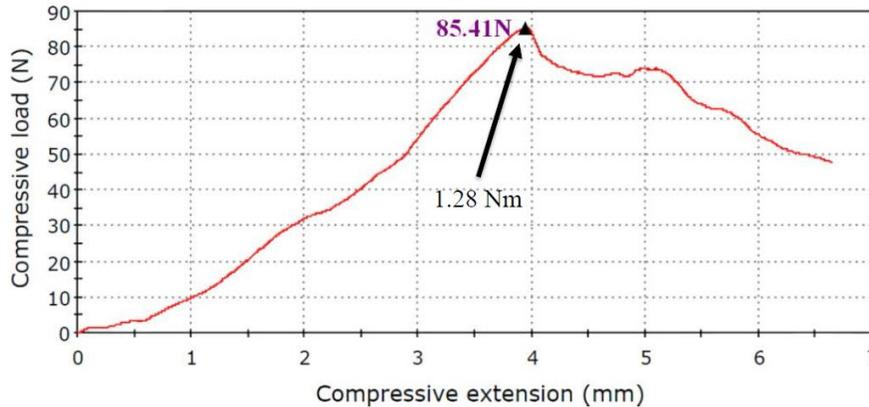
**Figure 3-73 Wrenching Strength Test with Cable in Fixture**
