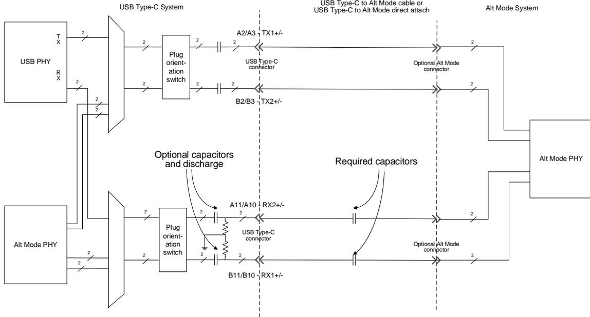
The USB Safe State is defined by the [USB PD](#) specification. The USB Safe State defines an electrical state for the SBU1/2 and TX/RX for DFPs, UFPs, and Active Cables when transitioning between USB and an Alternate Mode. SBU1/2 and TX/RX must transition to the USB Safe State before entering to or exiting from an Alternate Mode. Table E-1 defines the electrical requirements for the USB Safe State. See the [USB-PD](#) Specification for more detail on entry/exit mechanisms to the USB Safe State.
