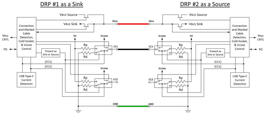
**CASE 2:** The following describes the behavior when a DRP is connected to another DRP. In this flow, the DRP #2 chooses to drive the random result to the opposite result using the [Try.SRC](#) mechanism.
