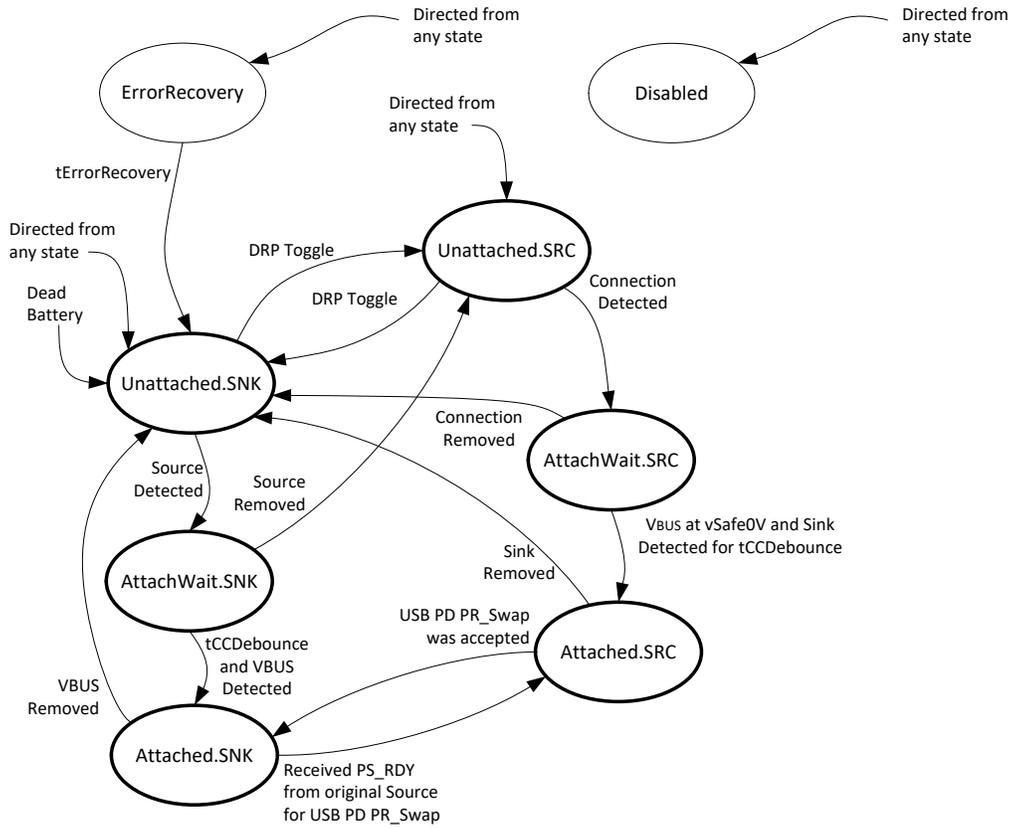
Figure 4-17 illustrates a connection state diagram for a DRP that supports Try.SNK and Accessory Modes.
