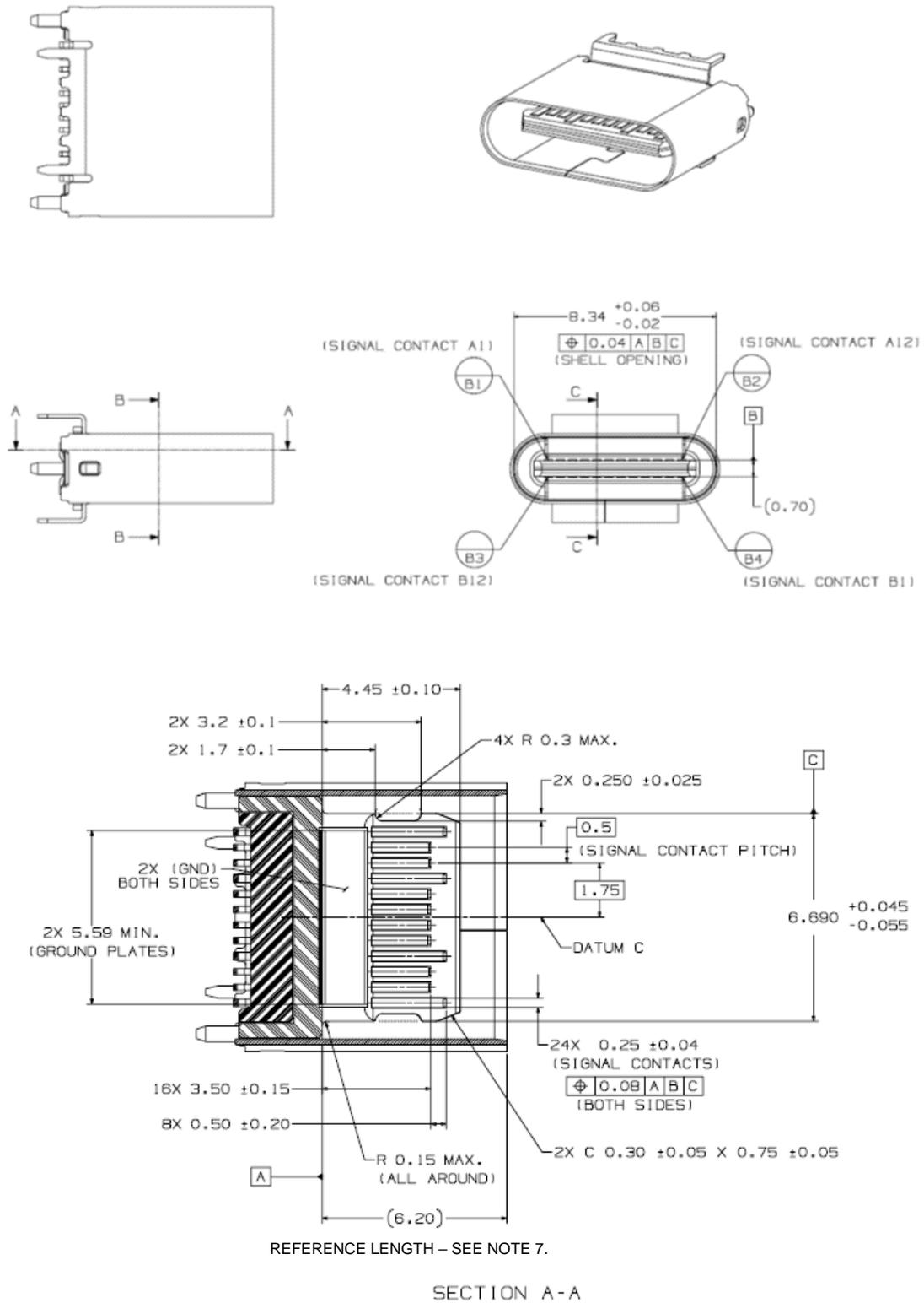
**Figure 3-1 USB Type-C Receptacle Interface Dimensions, cont.**
