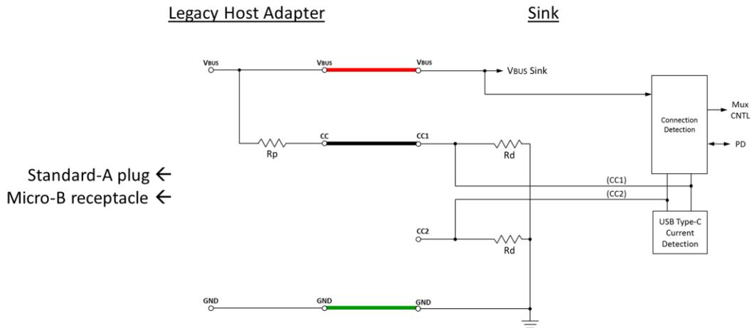
The following describes the behavior when a legacy host adapter that has an [Rp](#) to VBUS so as to mimic the behavior of a Source that is connected to a Sink. The value of [Rp](#) shall indicate an advertisement of Default USB Power (See Table 4-24), even though the cable itself can carry 3 A. This is because the cable has no knowledge of the capabilities of the power source, and any higher current is negotiated via [USB BC 1.2](#).
