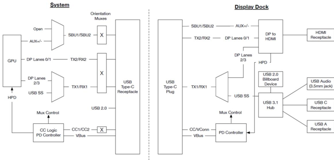
The system uses [USB PD](#) Structured VDMs to communicate with the dock to discover that it supports a compatible Alternate Mode. The system then uses a Structured VDM to enter the dock mode. Since [USB PD](#) is used, it may also be used to negotiate power for the system and dock. In this example, the SuperSpeed USB signals allow the dock to work as a USB-only dock when attached to a system that does not fully support the dock or even [USB PD](#).
