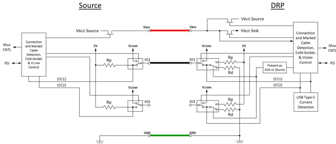
The following describes the behavior when a Source is connected to a DRP.
